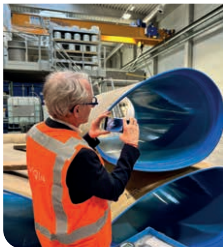
The shells are made from sand, fibreglass and resin, then placed in rotating moulds calibrated to the correct thickness.
